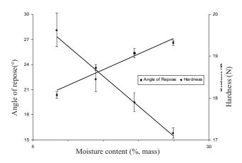
Fig. 4. Effect of moisture content on angle of repose and hardness.
