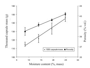
Fig. 2. Effect of moisture content on thousand capsule mass and porosity.
