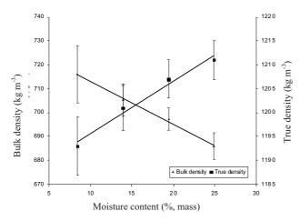
Fig. 3. Effect of moisture content on bulk and true density.
